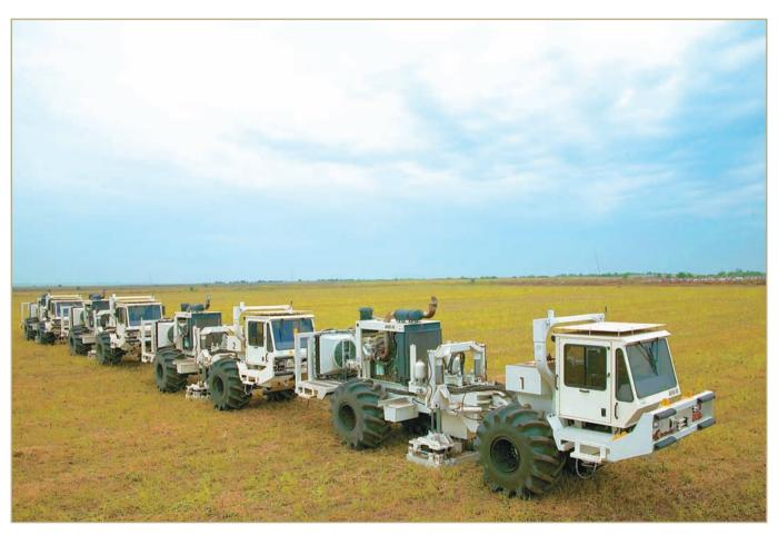
New generation seismic vibrators I/O AHV-IV 362 for 2-D and 3-D seismic research
