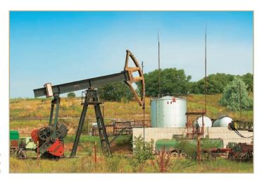
Prospecting drill-hole with deep pump for production
