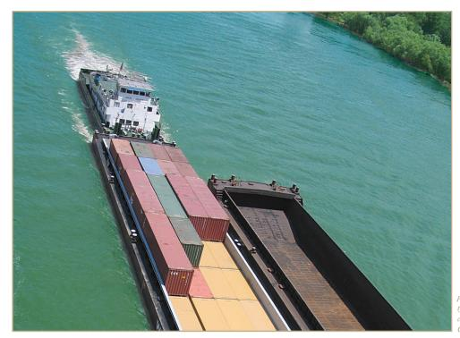
pushboat Georgi Izmirliev type with power 1 740 hp container transportation on the line
